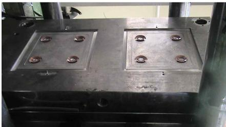
Fig. 9 Injection mold for experiment
