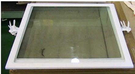
Fig. 10 Glass insert shelf for experiment
