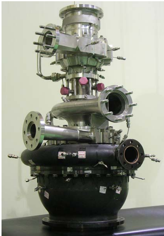
Fig. 2 Picture of turbopump assembly under test
