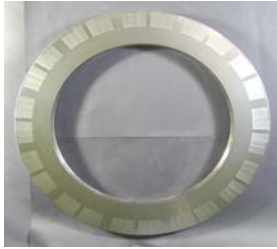
Fig.7 Sliding seal coated with TiCrN film
