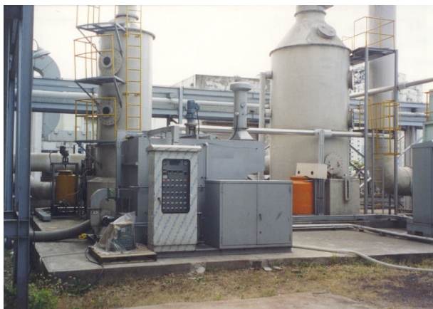
Figure 2. A photo of the pilot-scale biofilter installed in the pharmaceutical plant.
