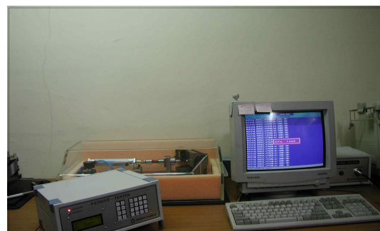
Fig. 3. Cyclic loading system.
