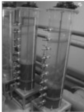
Fig. 4. Interfacial height for a various solids concentration with the polymer dosage at the settling time of 10 s(left) and 300 min(right) in Photograph.
