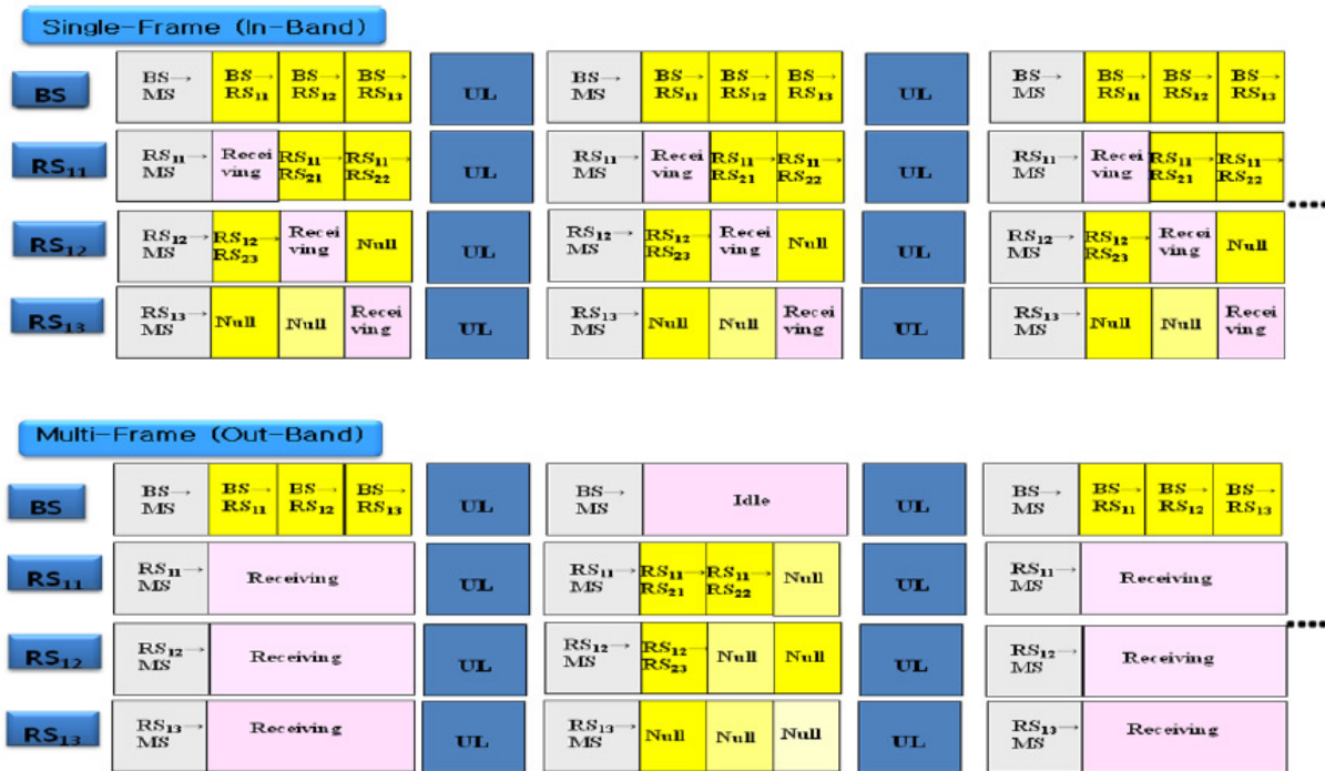
Figure 11. Frame transmission examples in the single-Frame Mode(Upper) and the multi-Frame Mode(Lower)
