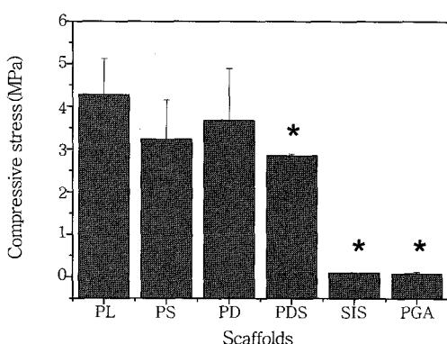
**Figure 1.** Compressive stress of various type scaffolds *in vitro*(PL; PLGA, PS; PLGA/SIS, PD; PLGA/DBP PDS; PLGA/DBP/SIS, SIS; SIS sponge, PGA; PGA nonwoven mesh, \* denotes significant difference with compared with PL, \*  $P < 0.05$ ).
