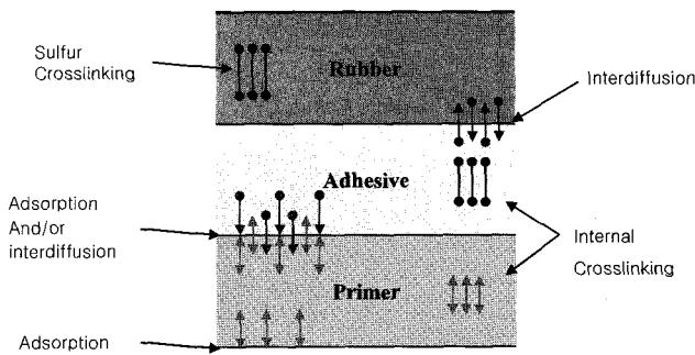
Figure 1. Adhesion of rubber and metal by adhesive.
