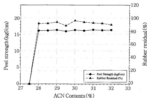
Figure 4. Peel strength and rubber residual of NBR/metal with respect to ACN contents ( $ML_{1+4}(125\text{ }^{\circ}\text{C}) : 46$ ).
