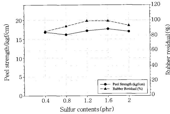
**Figure 7.** Peel strength and rubber residual of NBR/metal with respect to sulfur contents.
