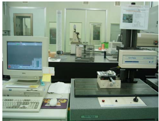
Fig. 3 Photograph of measuring instrument (Form Talysurf Series2)
