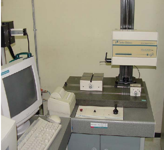
Fig. 3 Photograph of Fom Talysurf Series 2 set up for force measurement system
