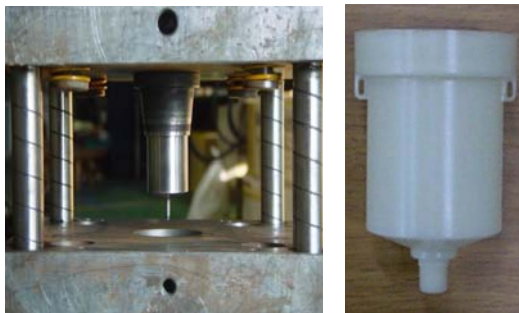
Fig. 13 The mold product of the body for automatic grease lubricator
