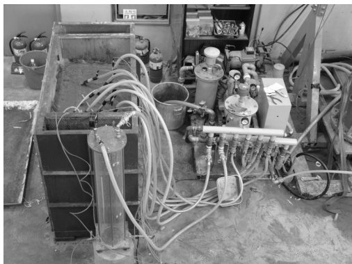
Fig. 3. PVD system installation setup
