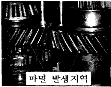
Fig. 2. Tribological vibration and noise by wear.
