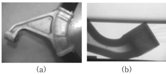
Fig. 8. The analysis of the complete product: (a) the blister test after heat treatment processing and (b) the result of X-ray test.
