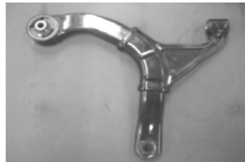
Fig. 9. The final product of the semisolid hybrid lower arm.
