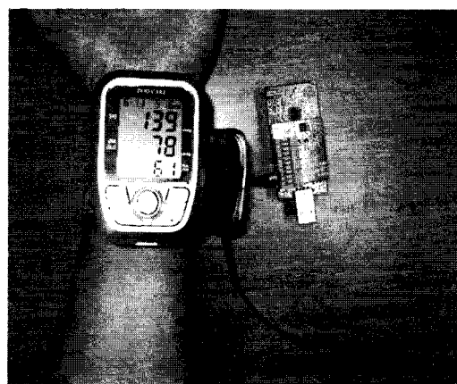
Fig. 2 Blood pressure and diabetes sensor node
