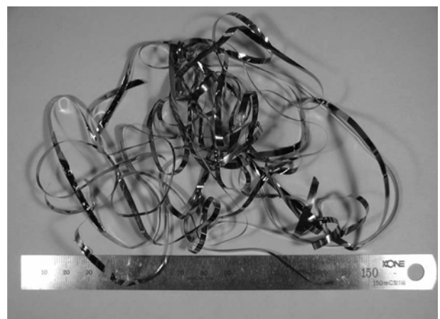
Fig. 1. As-spun ribbons fabricated at the wheel velocity of 55 m/s and the superheating temperature of 1500°C.
