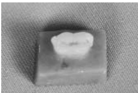
Fig. 4. Showing a fractured resin teeth specimen after strength test
