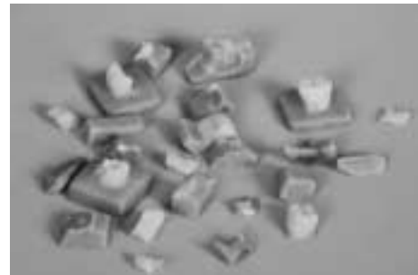
Fig. 3. Showing a fractured figure surface on the resin teeth specimens
