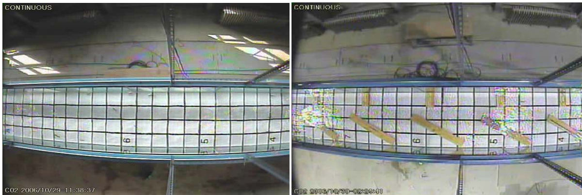
Fig. 5. With/Without Offset Baffles in Flume
