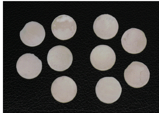
Fig. 2. Samples of Lava Frame Zirconia (Lt: After staining, Rt: Before staining).
