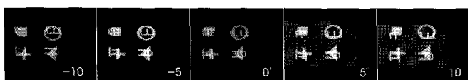
Fig. 9. The projection images of the phantom for various projection angles obtaining from the micro-CT system.
