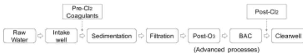
Fig. 1. Schematic flow diagram of the target water treatment system.
