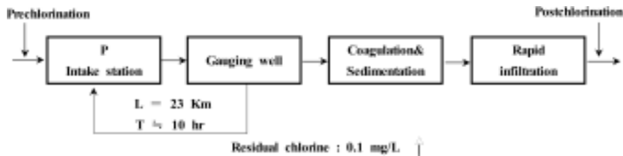
Fig. 1. Prechlorine and postchlorine injection points of water treatment process.
