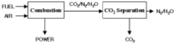
Fig. 2. Process diagram of post-combustion for CO 2 capture.
