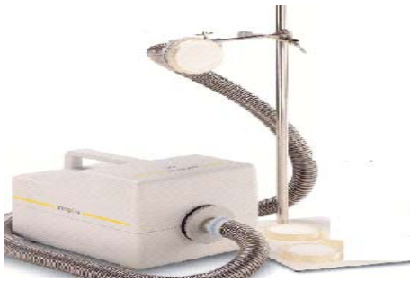
MD8 air scan air monitoring unit/ By Sartorius SKC Button Aerosol Sampler for inhalable dust sampling
