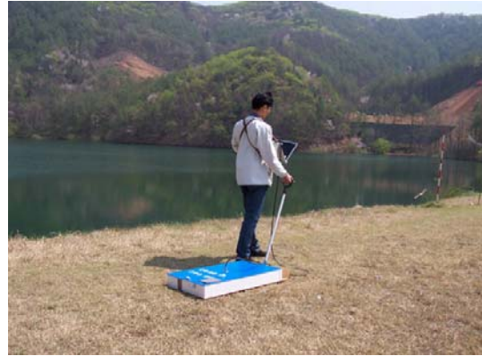
Figure 8. A surveyor pulling a GPR system to generate underground soundings [2]
