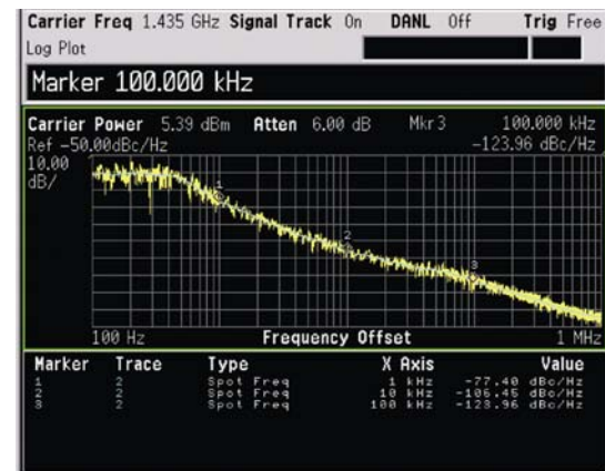
Figure 5. Measured phase noise performance of LO
