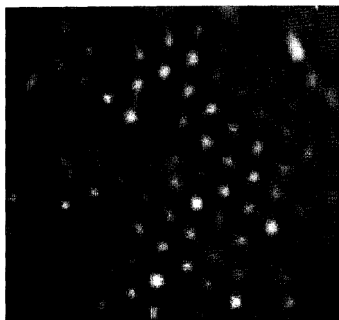
Fig. 2. STM image of the clean \text{Ni}_3\text{Al}(111) alloy surface. Tunneling parameters: size= (6.2 \times 7.7) \text{nm}^2 , I_t = 1.5 nA, U_B = 20 mV.
