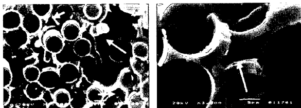
Fig. 2. Microstructures of SiC/SiC composite prepared by the conventional CVI process for 8 h. They show the closed pores from circumferential growth of deposits.
