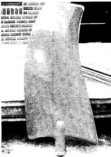
Fig. 8 Prototype of the axial F.R.P. fan.
