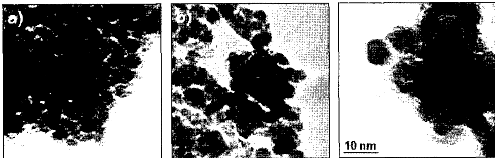
Fig. 3. TEM micrographs of FePt nanopowder synthesized with different reaction temperatures (a) 800°C, (b) 900°C and (c) 1000°C at 760 Torr by chemical vapor condensation process.
