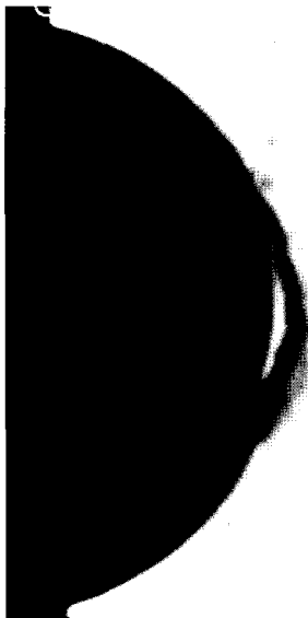
Fig. 16. V-shape notch around the opening from CT image
