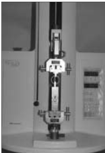
Fig. 2. Measurement of microtensile bond strength on universal testing machine.
