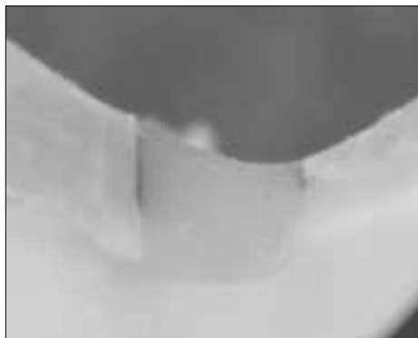
Fig. 6. Score 2 of dye penetration.
