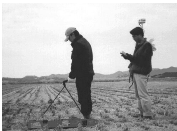
Fig. 3. Field measurement of electrical conductivity by EM 38 and GPS (Jung et al., 2002).
