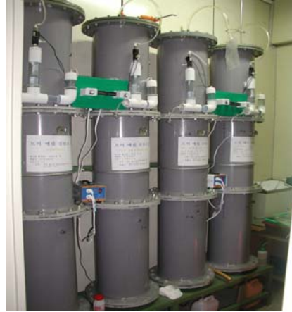
[Fig. 1] Schematic of the anaerobic lysimeter. (unit : cm)
