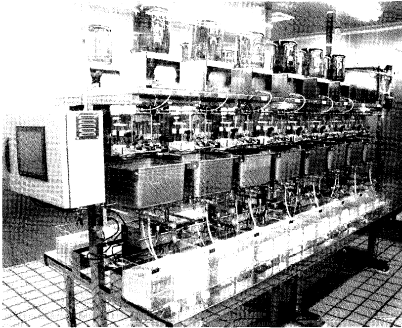
Fig. 2. An automatic flow-through exposure system used in this experiment.
