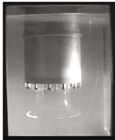
[그림 9] Observation of the vortex formation in the preliminary test. (LLWL, Rated, AEV)
