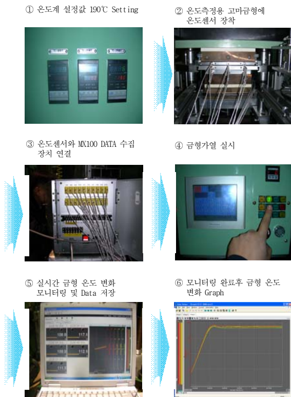
Fig. 7 Test procedure of mold temperature distribution.
