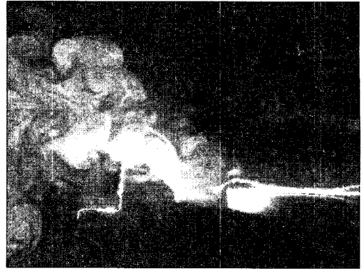
Fig. 6 Flow visualization around the guide wall by using PIV
