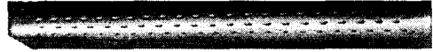
Fig. 6 1st bucket leading edge cooling hole damage of MS7001FA+ and MS7001FA+e model
