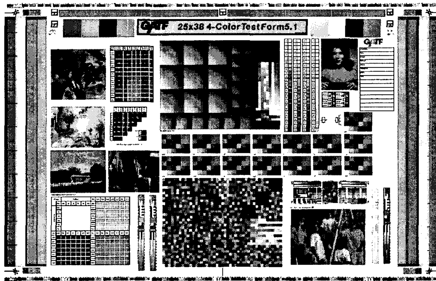
Fig. 1. GATF/ The 25 × 38 Sheetfed Test Form 5.1.
