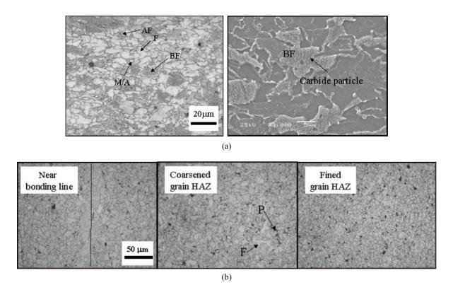
Fig. 3. Microstructure of base metal and weld joint; (a) Base metal, (b) Weld joint
