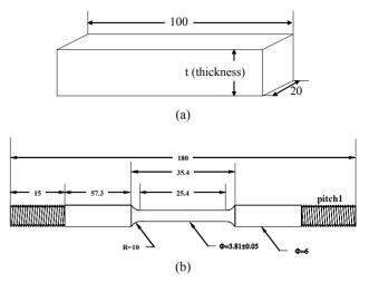
Fig. 1. Schematic of specimen for HIC and SSC tests; (a) HIC, (b) SSC
