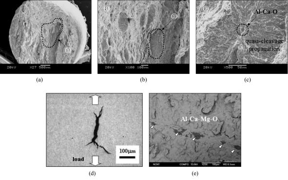
Fig. 8. SSC nucleation and propagation of base metal; (a) Fracture surface, (b) and (c) Nucleation of cracks perpendicular to load axis, (d) A cross-section showing typical SOHIC, (e) SOHIC nucleation at an oxide cluster and single oxide inclusion
