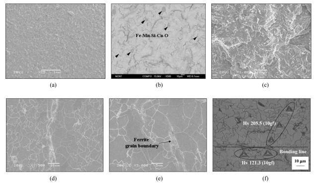
Fig. 7. HIC nucleation and propagation of weld joint; (a) Fracture surface, (b) HIC nucleation at a lot of oxide-inclusions, (c) HIC propagation in quasi-cleavage manner, (d), (e) and (f) HIC propagation path
