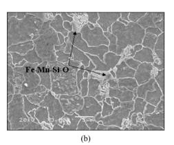
**Fig. 4.** Species of inclusion in base metal and nearby bonding line of weld joint; (a) Base metal, (b) Bonding line of weld joint
