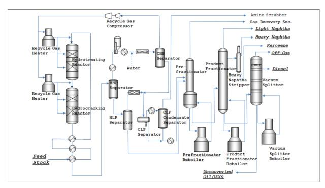
Fig. 1. Simplified PFD of hydrocracking unit
