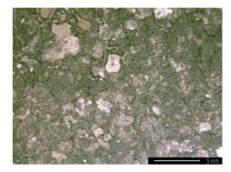
Fig. 9. Tube Inside Scale Sample
