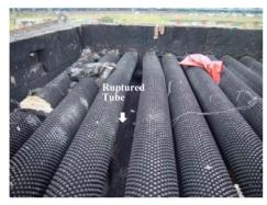
Fig. 4. Appearance of the failed convection module after dissecting
