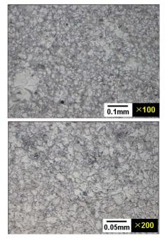
Fig. 11. Tube base metal microstructure
