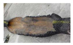
Fig. 6. Ruptured tube appearance after dissecting
