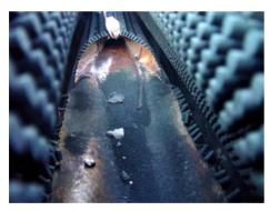
Fig. 5. Appearance of the ruptured tube in situ
