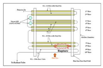
Fig. 3. Side view drawing of convection zone tube configuration
