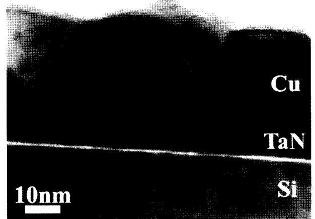
Fig. 2. Cross sectional TEM image of sample Cu 20 nm/ALD TaN 10 nm/Si (Reused with permission from Y. Y. Wu, A. Kohn, and M. Eizenberg, Journal of Applied Physics, 95, 6167 (2004). Copyright 2004, American Institute of Physics (Ref. 4)).
