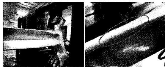
Fig.15 Crack in roll durability test of tubular torsion beam by stamping
