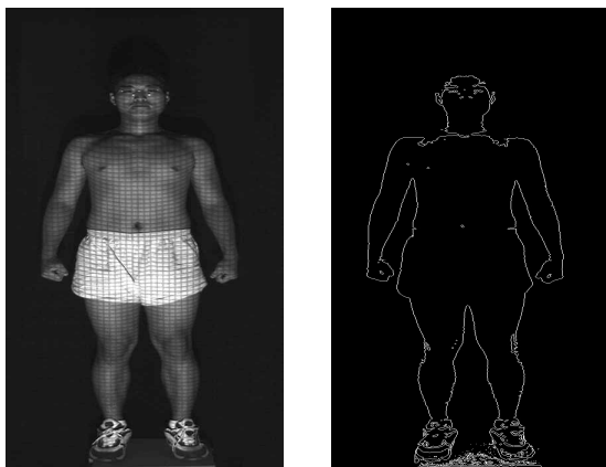
(a) 원영상 (b) 외곽선 추출 (a) Original image (b) Contour line extraction
