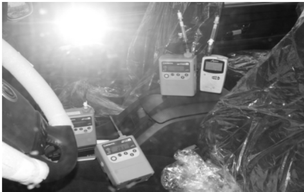
Figure 1. VOC sampling from inside of new vehicle.
