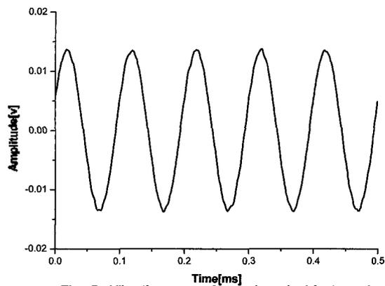
Fig. 7. Vibration wave from piezoelectric transducer.
