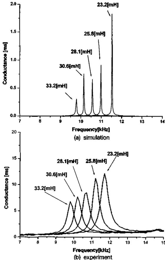
Fig. 4. Resonance frequency change by inductance variation.
