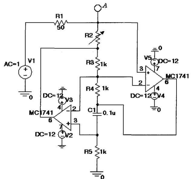
Fig. 2. PSpice equivalent model for electronic inductance.
