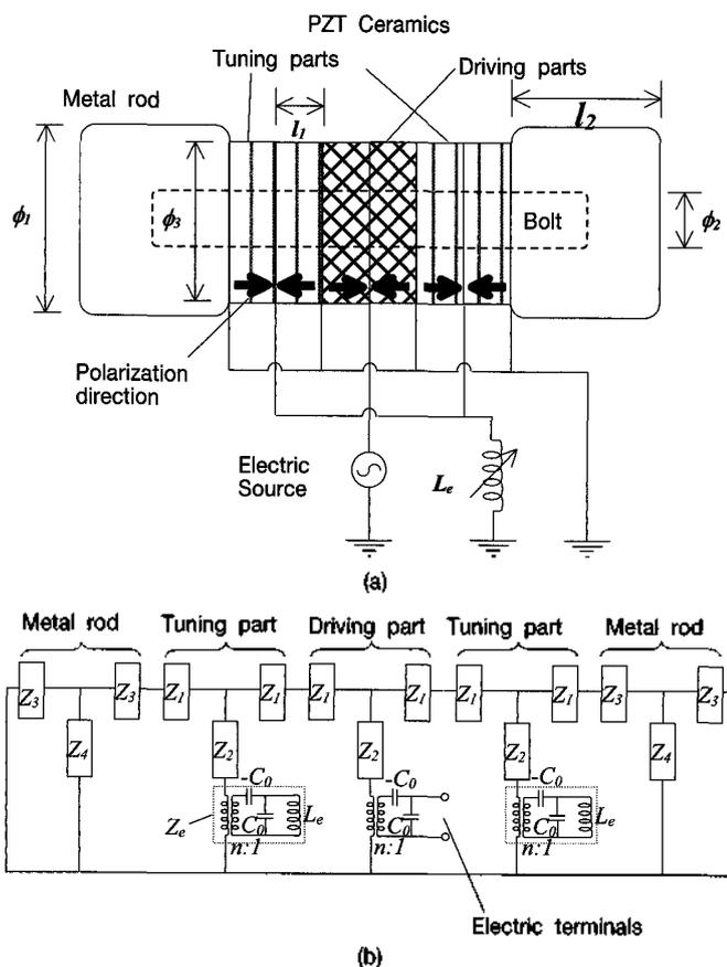
Fig. 1. Construction and equivalent circuit of frequency controllable transducer.
