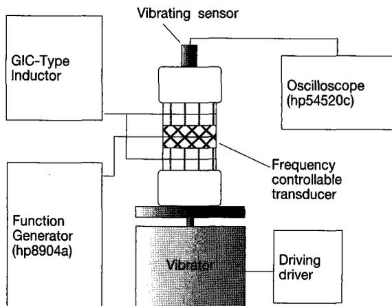
Fig. 5. Experimental setup for active vibration control.
