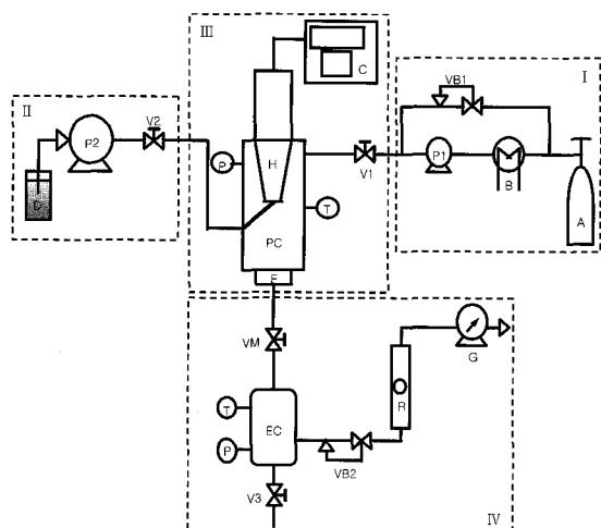
**Figure 2.** Schematic representation of our SAS apparatus. A,  $\text{CO}_2$  siphon tank; B, cooler; C, ultrasonic generator; D, polymer solution; F, steel frit; G, wet gas test meter; H, horn of ultrasonicator; P, pressure gauge; T, temperature gauge; R, rotameter; P1 and P2, high pressure liquid pumps; VB1 and VB2, back pressure regulator; V1, V2 and V3, control valves; VM, micro-metering valve; PC, precipitation chamber; EC, expansion chamber.
